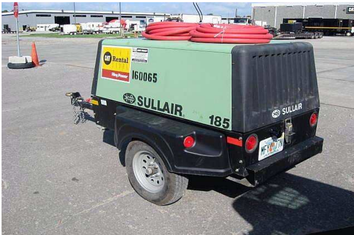
COMPRESSOR AND HOSES FOR PNEUMATIC DRILLS AND HAMMERS TO WORK INSIDE THE MINE
