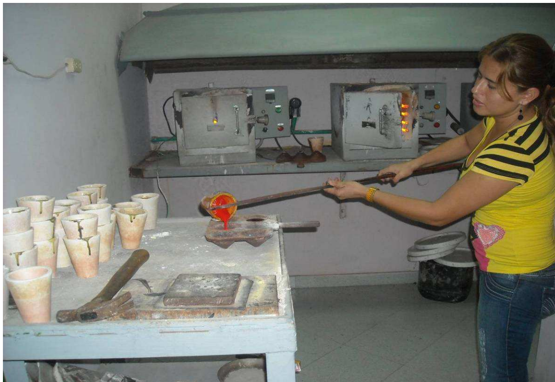
POURING MOLTEN GOLD & SILVER ORE AT EL GUAMO FOUNDRY INTO GRAPHITE CONTAINERS
