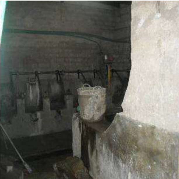
BALL MILLS USED TO MAKE THE GOLD & SILVER ORE A FINE POWDER FOR THE FINAL PROCESS
