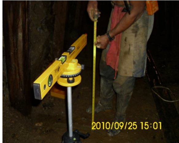
Mona Minas S.A. Miners at work in front of the mine entrance! The laser guided level being used to keep the mine shaft floor level. Our site team leader Ramon sets the charges for the next blast!
