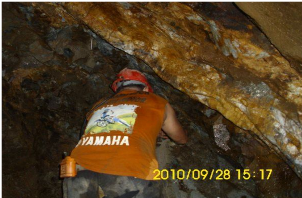
MONSTER VEIN EXPOSED ABOVE RAMONS HEAD THE OXIDATION IS EVIDENT
